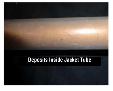
Without TWT® treated and conditioned water, the pipe & jacket tube (heat exchanger) filled with calcium deposits.
